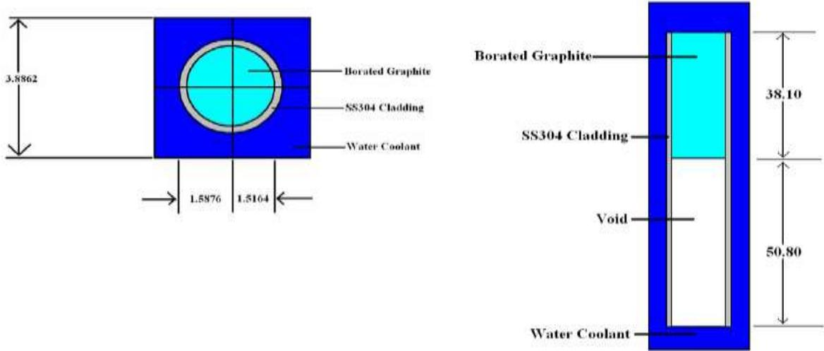
Figure 4: Cross-sections of the transient rod with dimensions (in cm) and materials
