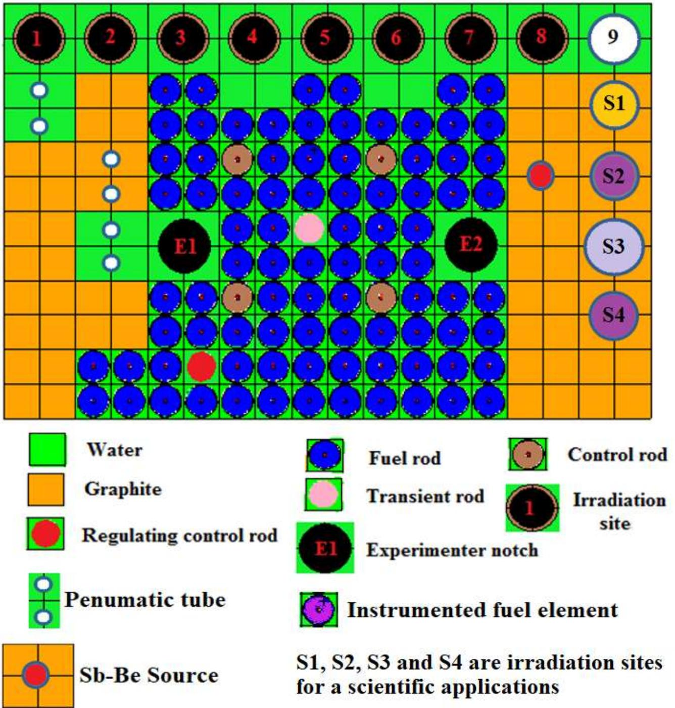
Figure 6: Cross-sections of the TRIGA-1MW reactor using MCNP5-beta code.
