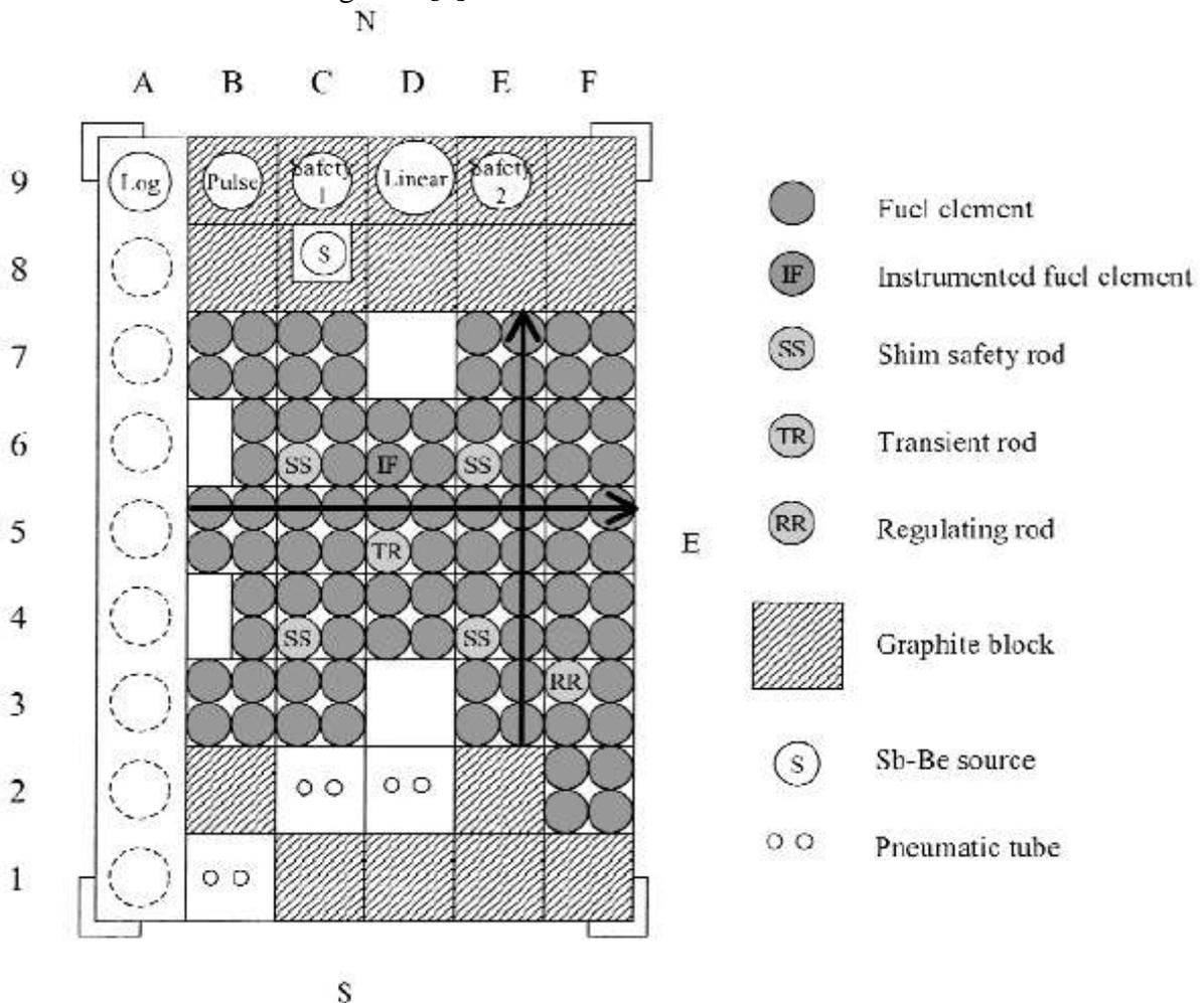
Figure 1: TRIGA-1MW reactor core, that is located in the NSCR.
