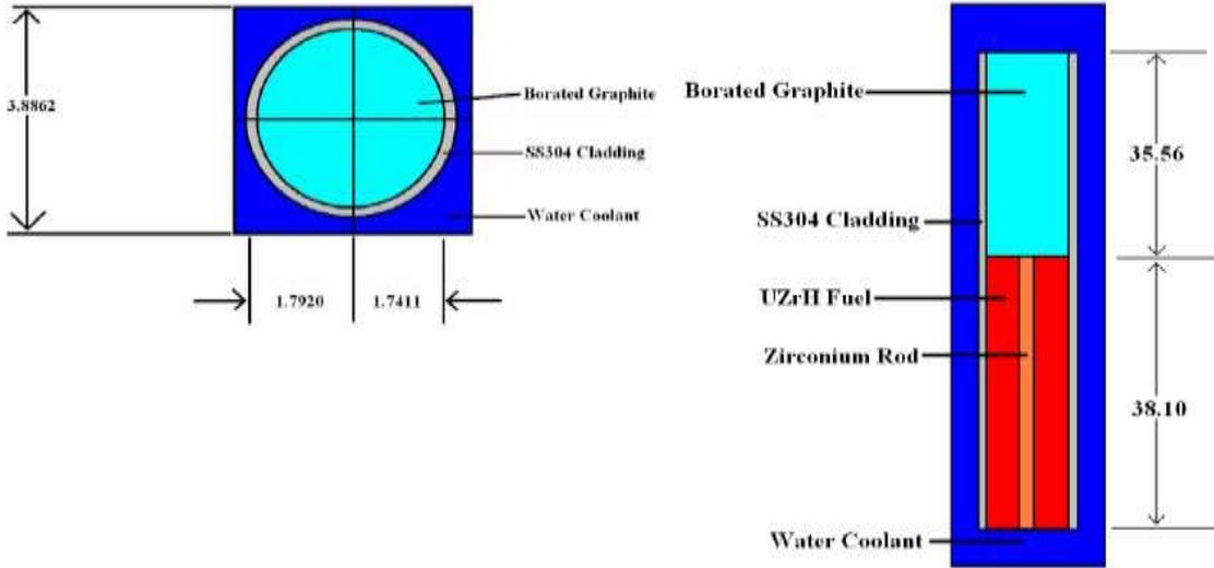
Figure 3: Cross-sections of the shim safety (control) rod with dimensions (in cm) and materials
