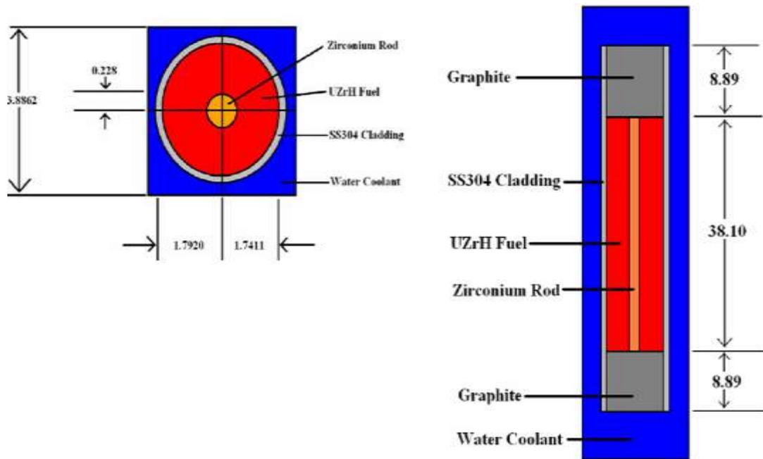
**Figure 2: Cross-sections of the fuel element with dimensions (in cm) and materials**
