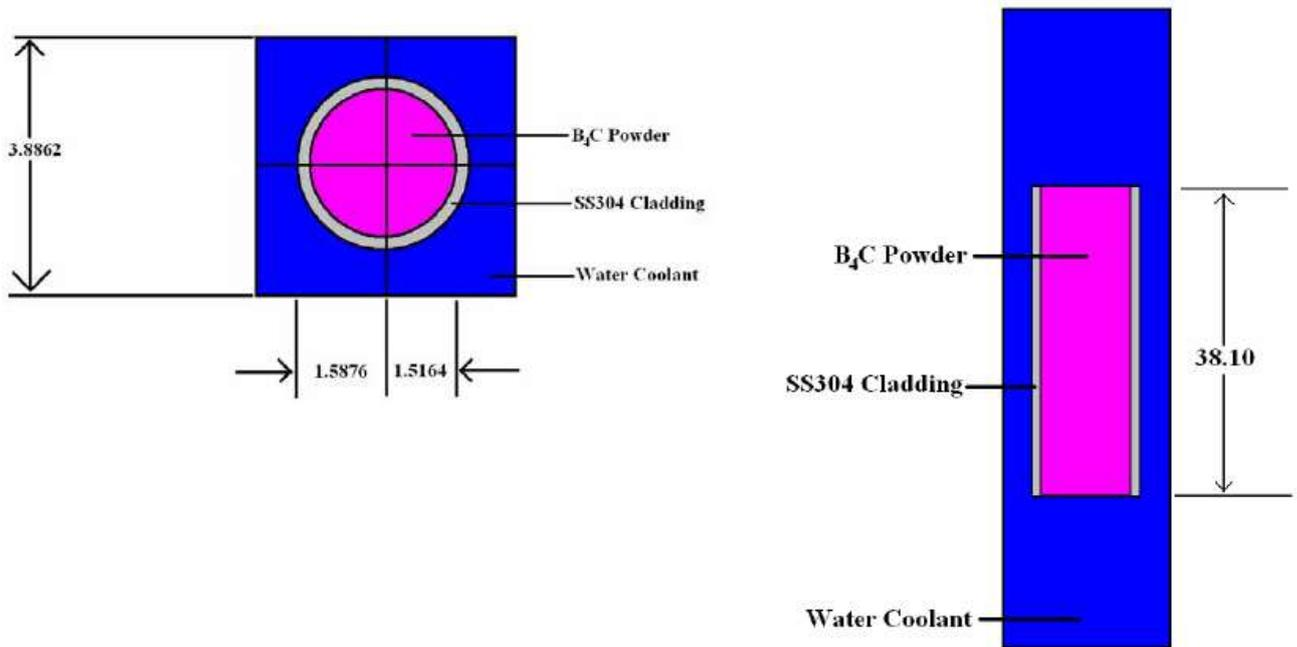
Figure 5: Cross-sections of the regulating control rod with dimensions (in cm) and materials
